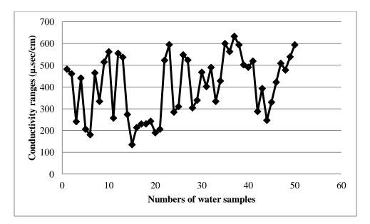
Figure 15 : Conductivity EC Values of 50 RWH samples
