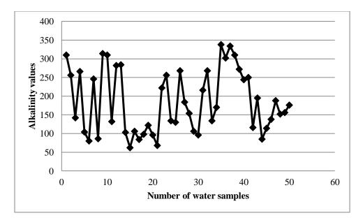
Figure 19 : Alkalinity Values of 50 RWH samples
