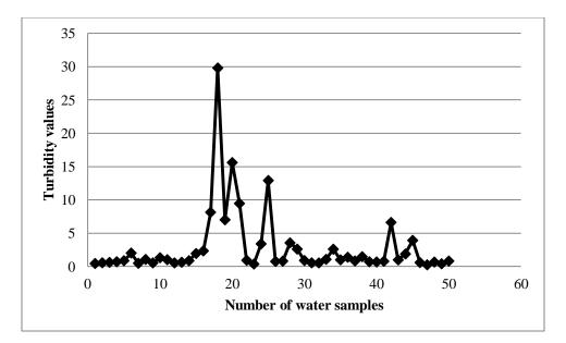
Figure 17 : Turbidity Values of 50 RWH samples
